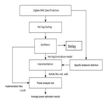
Figure 6: Algorithm used to obtain the power and delay results in Xilinx ISE tool
