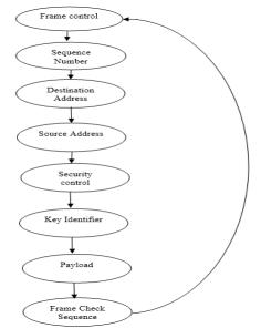
Figure 5: Algorithm used for ZigBee MAC transmitter design
