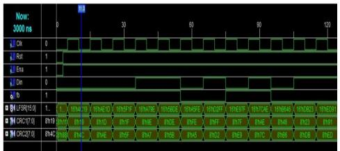
Figure.8 CRC Simulation Waveform
