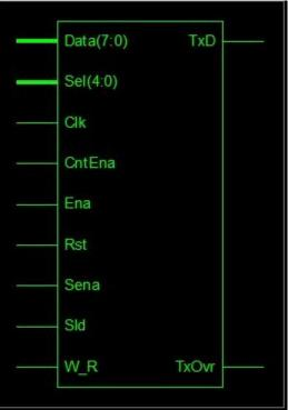
Figure.9 RTL schematic of ZigBee transmitter
