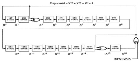
Figure.4 CRC-16 Generating circuit
