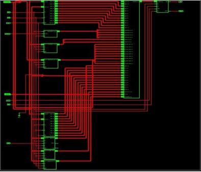
Figure.10 RTL schematic of ZigBee transmitter
