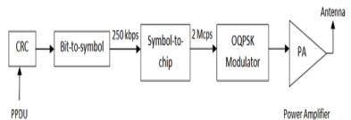
Figure.6: Detailed architecture of the proposed digital transmitter.
